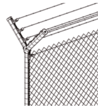
ADDITIONAL DOUBLE INCLINED EXTENSION BRACKET WITH BARBED WIRE (ONLY FOR LUX-80 TUBE)
