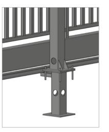
2. With double base plate system: anchorage via double-founded base plates system.
