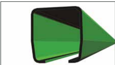
1. LOWER GUIDE: guidance system for the cantilever carriages to ensure that the gate slides perfectly.
